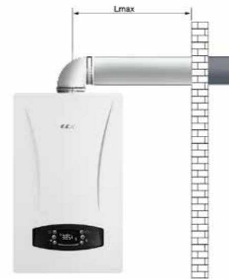
Horizontal Hermetic Flue Application
