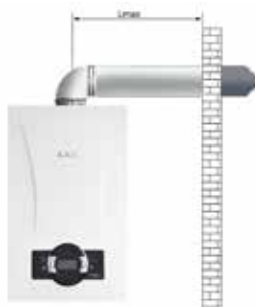
Horizontal Hermetic Flue Application L max. distance with single elbow: 10 m, Ø60/100 L max. distance with single elbow: 20 m, Ø80/125
